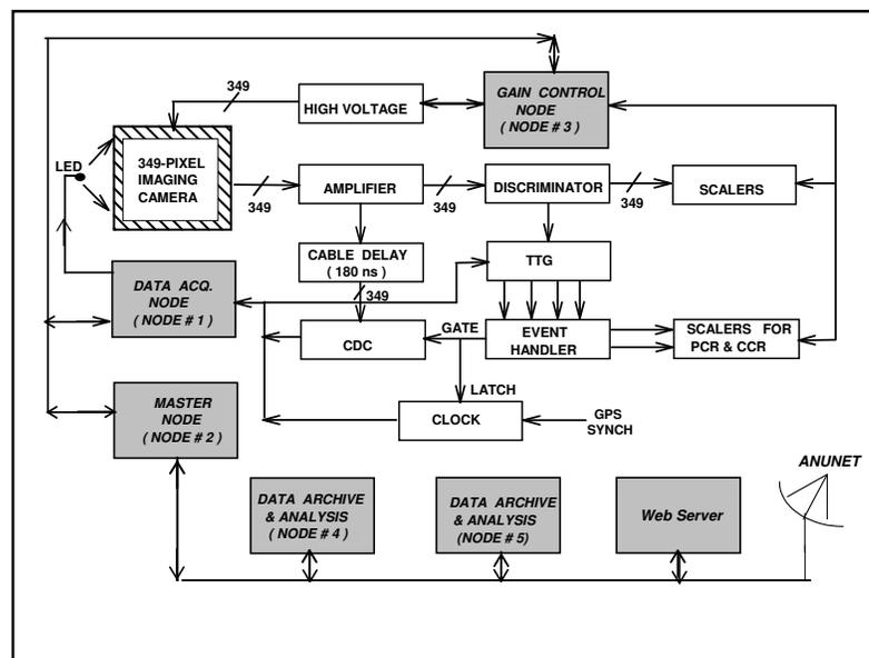
**Figure 1.** Block diagram of the back-end signal processing electronics used in the TACTIC imaging element; TTG:TACTIC Trigger Generator; PCR: Prompt Coincidence Rate; CCR: Chance Coincidence Rate.
