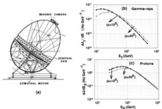
**Figure 1.** (a) A schematic of the MACE gamma-ray telescope planned to be set up at Hanle. (b) Differential detection rate for gamma-rays as a function of the primary energy. (c) Differential detection rate for protons as a function of the primary energy.
