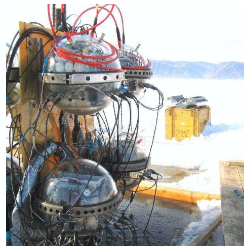
Figure 4. NT200+ central DAQ electronics in its pressure housings, before deployment. Upper spheres are underwater PC-NT200 and PC-NT+, detailed in Fig.3.
