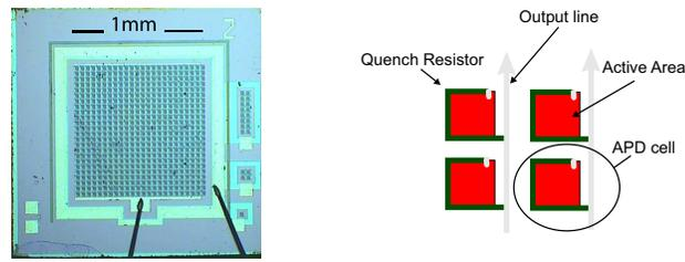
**Figure 1.** The left picture shows a 576 cell SiPM with a total sensor size of  $1 \times 1 \text{ mm}^2$ . On the right hand side an exemplary view of four Geiger-APD cells is shown which are part of a SiPM (c. f. text for further explanation).
