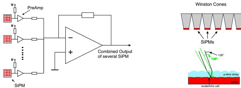
**Figure 3.** Concept of a possible application of a  $5 \times 5 \text{ mm}^2$  SiPM in IACTs. On the left side, a readout is sketched which combines several SiPMs to one output channel. On the right side, two possible methods are sketched by which the effective active area can be increased.
