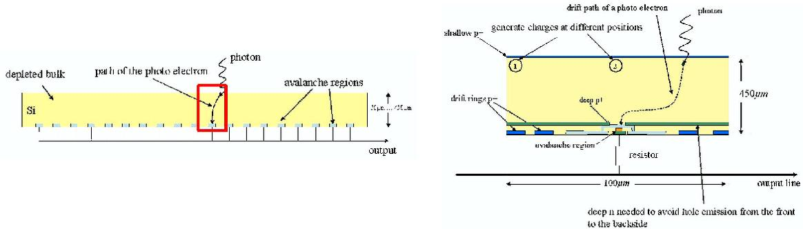
**Figure 2.** Schematic view of the back illuminated SiPM under investigation by the HLL. On the left side, a cross section through a back illuminated SiPM is sketched. On the right side, a blow-up of a single SiPM cell is shown. The drift path of a virtual photo electron from its point of generation until it reaches the Geiger APD is added.
