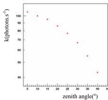
**Figure 3.** The minimum signal intensity  $k$  as a function of zenith angles
