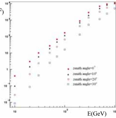
**Figure1.** The  $A_{\text{eff}}$  of ARGO for gamma-rays from different zenith angles, as a function of primary energies
