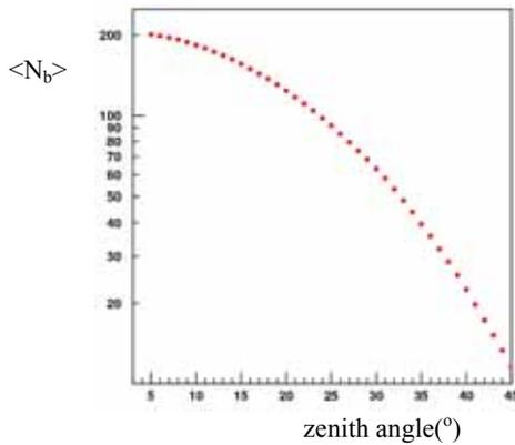
**Figure 2.** The background rate  $\langle N_b \rangle$  within  $1\text{s}$  as a function of zenith angles
