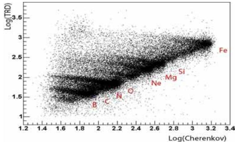
**Figure 3:** Measurements of the energy deposited in the TRD tubes versus the normalized Cherenkov light signal during the flight ( $\sim 1$  day).
