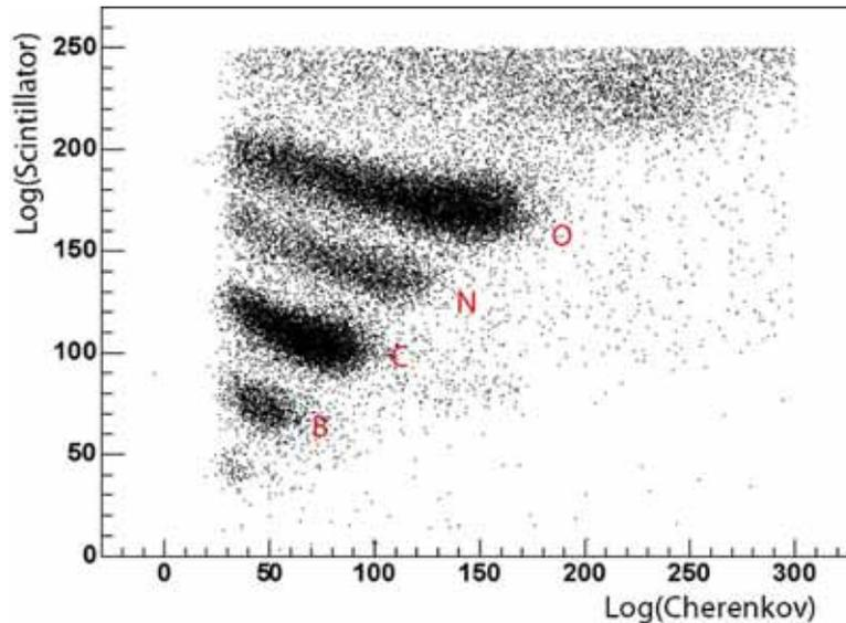
**Figure 2.** Measured energy losses in the TCD scintillator versus Cherenkov light signal for a short ( $\sim 1$  day) portion of the flight. B,C,N and O nuclei populations are clearly visible.
