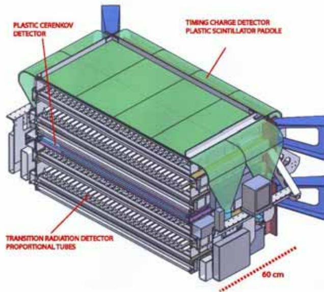
**Figure 1.** A mid cross-section of the CREAM TRD/TCD/Cherenkov detectors. The overall detector is  $1.2\text{m} \times 1.2\text{m}$  square.
