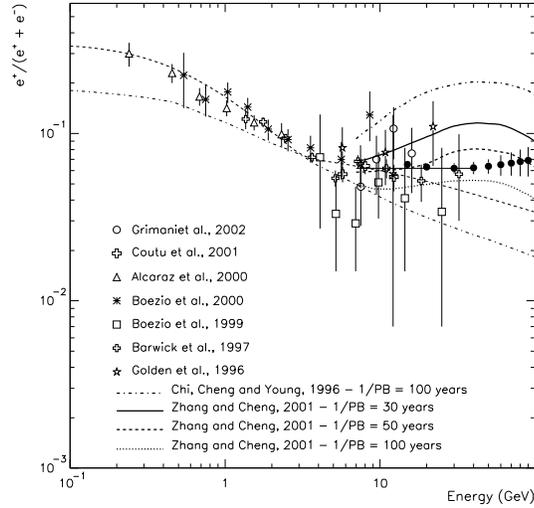
**Figure 1.** Positron fraction measurements in cosmic rays carried out during the last decade [13]. Thin dashed and dot-dashed lines represent the calculated secondary  $e^+/(e^+ + e^-)$  reported in [5] and [6], respectively. See text for additional details.
