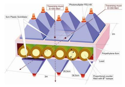
Figure 2 Nor Amberd Multidirectional Muon Monitor (NAMMM)
