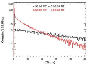
**Figure 3.** Histogram of time intervals between successive neutron counts, as measured by special instrumentation operated during the 2004-2005 Bartol/Tasmania latitude survey. The black (flatter) curve represents a Galactic spectrum, while the red curve includes the peak of the GLE. By modeling these time histograms, we hope to gain new information on the spectrum of the GLE.
