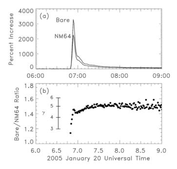
**Figure 2.** (a) Count rate of NM64 and polar bare neutron counters at South Pole during the January 20, 2005 GLE, expressed as a percentage of pre-event background. These data have now been normalized to sea level using two attenuation lengths [6], and hence display a somewhat smaller increase than that shown in Figure 1 or Table 1. (b) Ratio of polar bare to NM64, together with implied spectral index  $\gamma$  for an assumed power law in rigidity.
