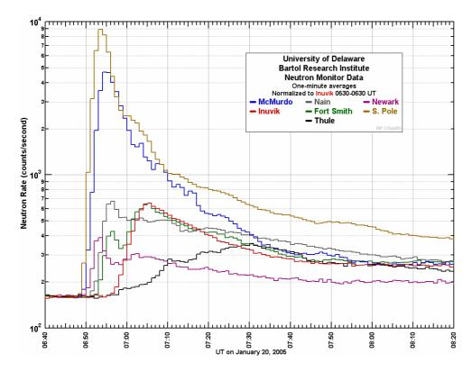
**Figure 1.** On January 20, 2005 the Sun emitted cosmic rays of sufficient energy and intensity to increase radiation levels on Earth's surface. The GLE was especially intense at South Pole (highest peak) and McMurdo, Antarctica (second highest), where radiation levels increased by factors of 56 and 30, respectively, in a span of 5 minutes. The McMurdo increase was the largest observed at sea level since 1956.
