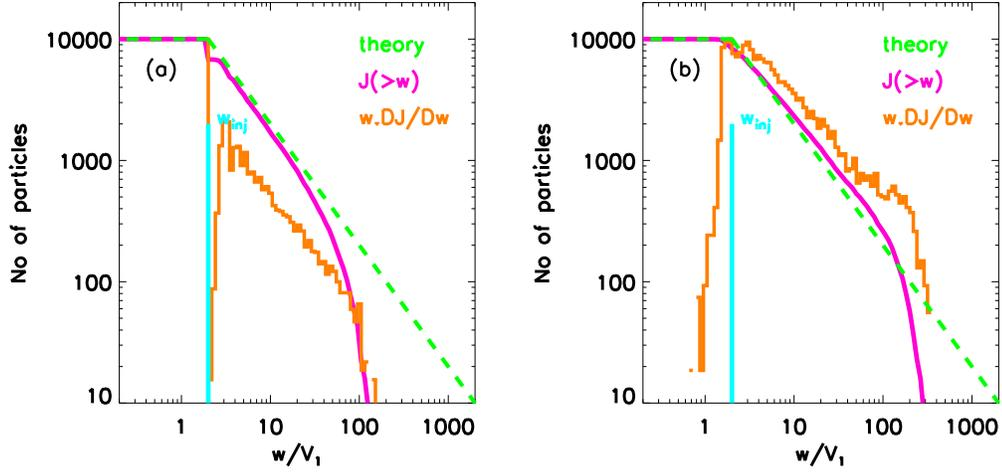
**Figure 2.** Comparison of acceleration efficiency for a parallel shock only (a) and that with a deflection behind the shock (b). Dashed lines indicate predictions of standard diffusion theory
