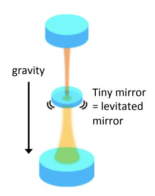
Schematic of the sandwich type optical levitation.
