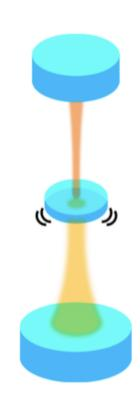
Schematic of the sandwich type optical levitation.
