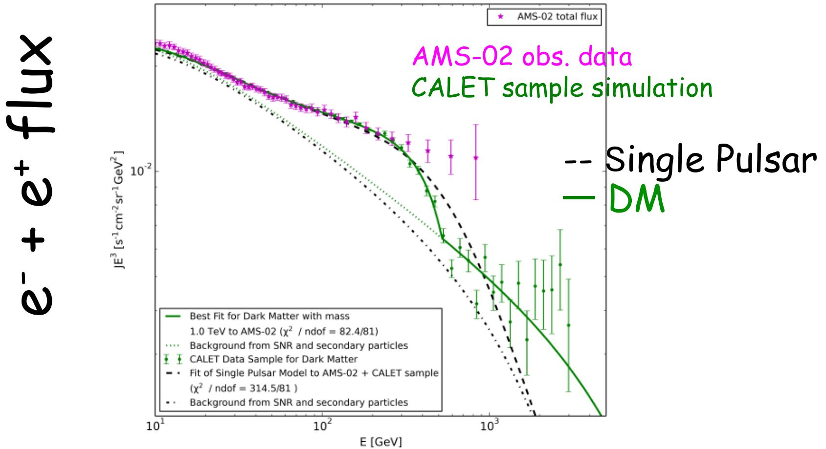
Decaying DM $\rightarrow\mu\mu\nu$ : 73% and eev: 27% with  $m_{\text{DM}} = 2 \text{TeV}$
