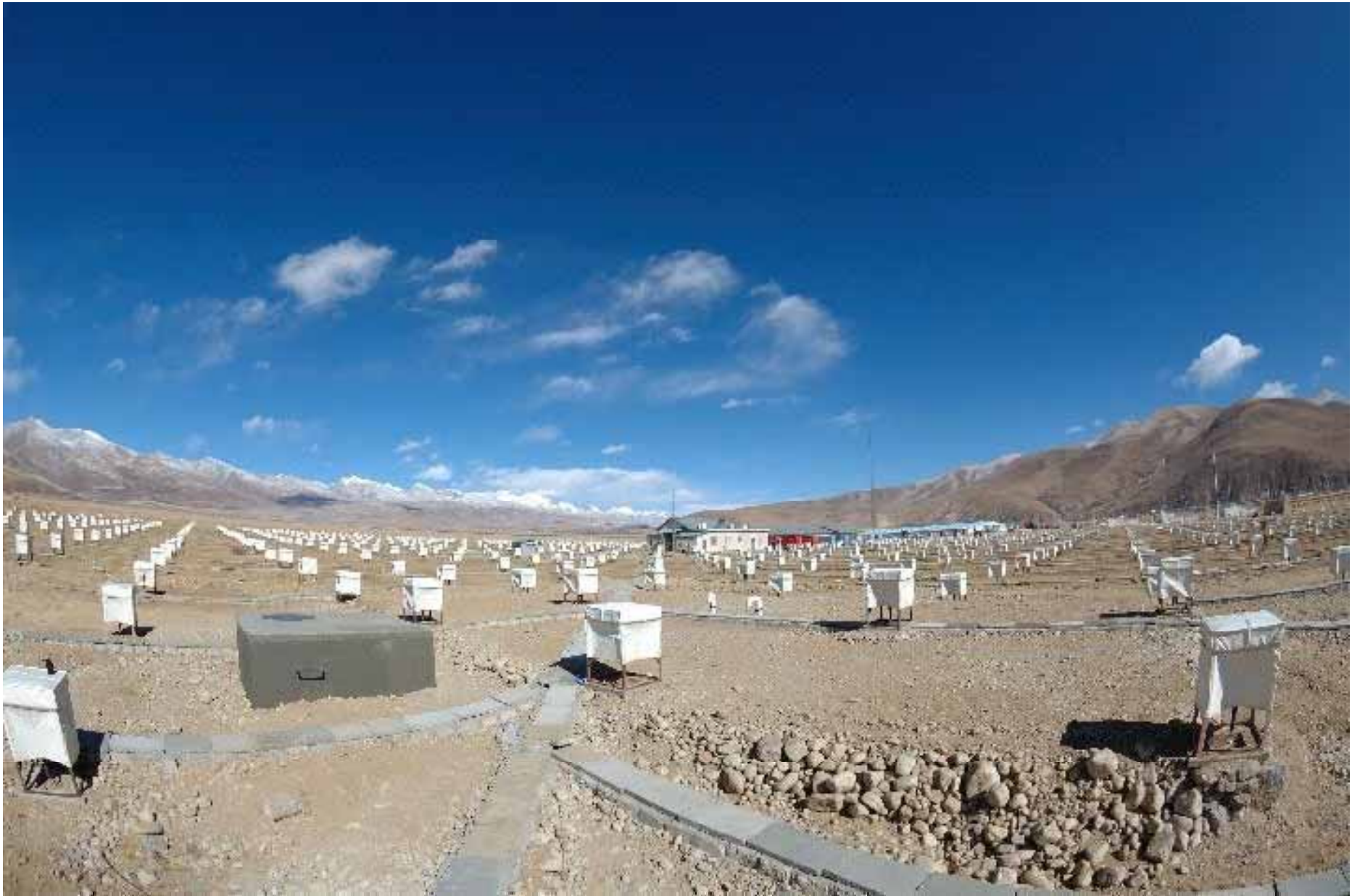
Prototype Muon Detector after backfilling
