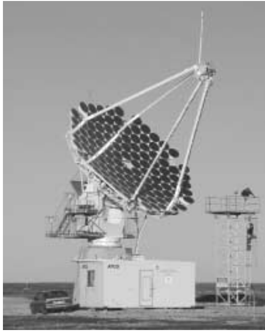
FIGURE 1. The 10 m telescope completed in February 2000 in Woomera, South Australia. The reflector consists of 114 spherical mirrors of 80 cm radius. The imaging camera is set at the focus ( f = 8 m) and can be accessed from the tower (right) for maintainance.
