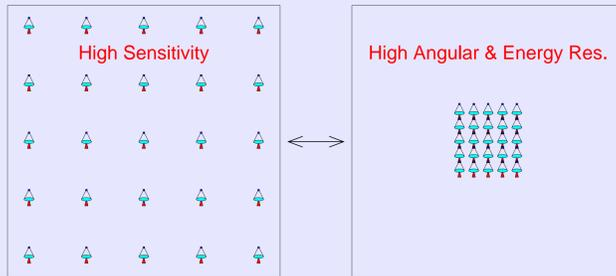
Figure 3: Two major configurations of the “Mobile Telescope Array” considered as an extension plan of TenTen.
