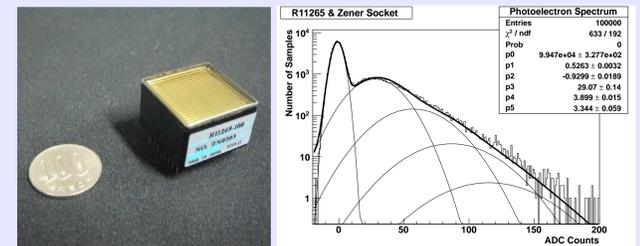
Figure 7: Left: Hamamatsu R11265 PMT (1 inch square, super bialkali photocathode, 12 stage metal channel dynode) planned to be used for test observations. Right: photoelectron spectrum of a R11265 PMT measured with a Zener socket, illuminated by a blue LED. The fitted model is a convolution of Poisson and Gaussian distributions.
