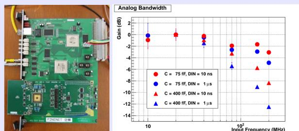
Figure 4: Left: test setup of a prototype AMC board. The AMC board at the bottom is connected to the module for readout. The AMC ASIC chip is located in the left-hand side of the AMC board. Right: result of analog bandwidth measurements of the AMC board.
