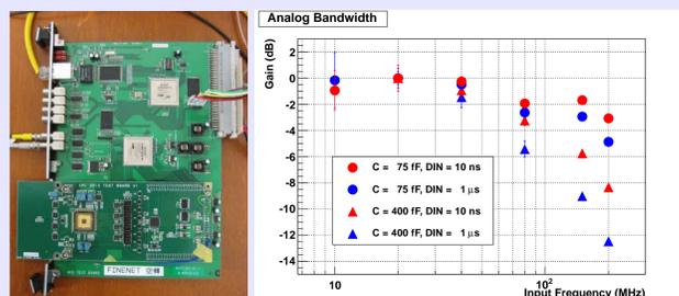
Figure 4: Left: test setup of a prototype AMC board. The AMC board at the bottom is connected to the module for readout. The AMC ASIC chip is located in the left-hand side of the AMC board. Right: result of analog bandwidth measurements of the AMC board.
