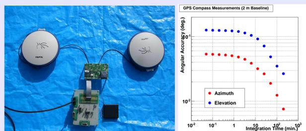
Figure 5: Left: GPS compass board (Hemisphere Crescent Vector OEM) and GPS antennas (Novatel GPS-701-GG) used for test measurements. Right: accuracies of direction measurements as a function of the integration time.
