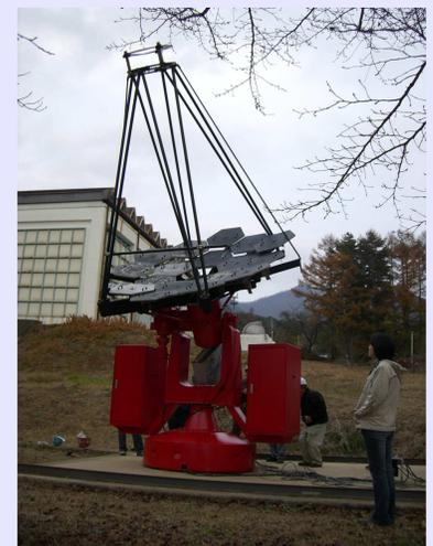
Figure 6: 3 m diameter Cherenkov telescope installed at the Akeno Observatory of ICRR.
