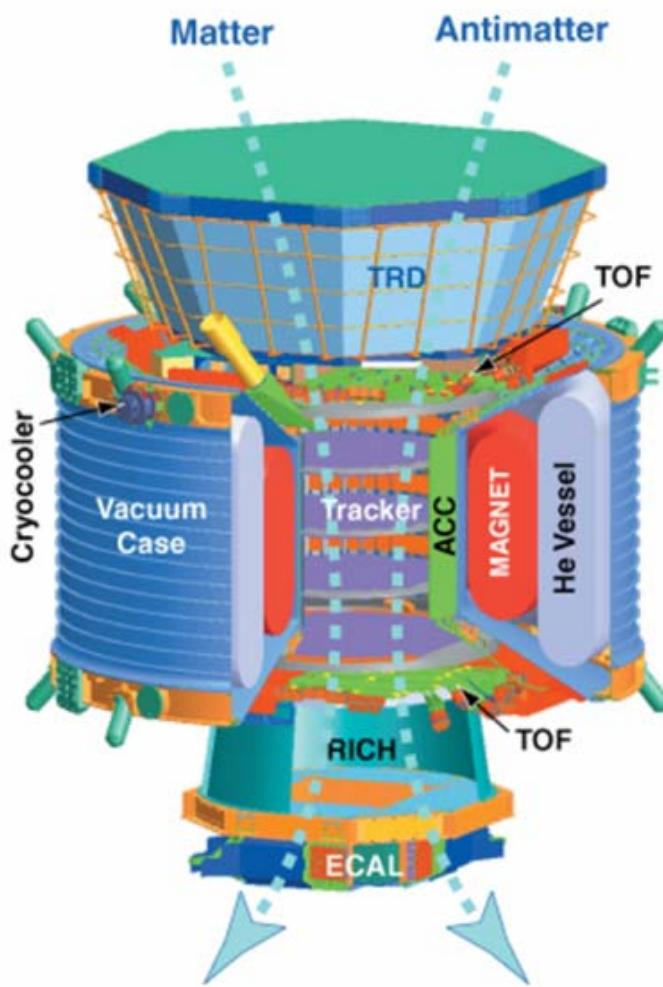
300,000 channels of electronics  $\Delta t = 100 \text{ ps}$ ,  $\Delta x = 10\mu$
