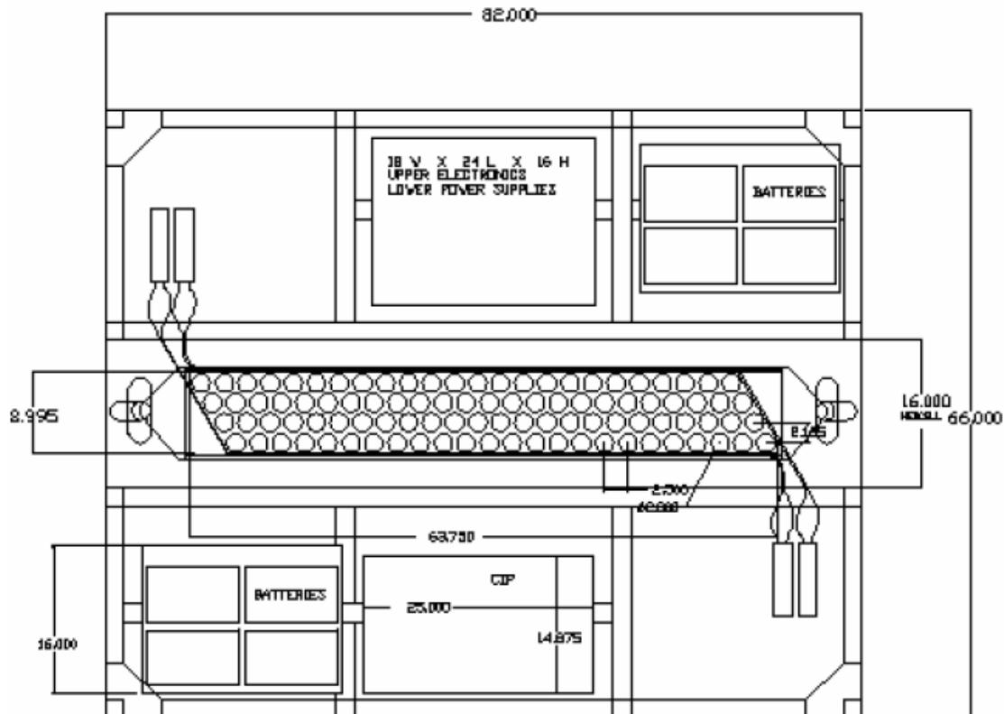
Figure 3. The CREST-1 instrument (dimensions in inches)
