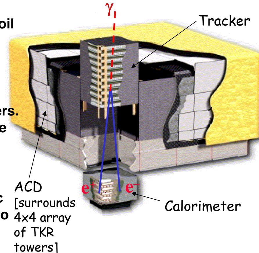
Systems work together to identify and measure the flux of cosmic gamma rays with energy 20 MeV - >300 GeV.
