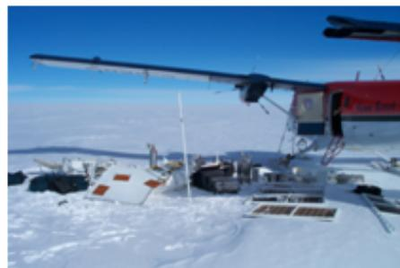
ATIC is designed to be disassembled in the field and recovered with Twin Otters. Two recovery flights are necessary to return all the ATIC components. Pictures show 1<sup>st</sup> recovery flight of ATIC-1
