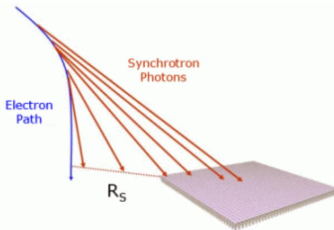
CREST will detect high-energy electrons by measuring the X-ray synchrotron photons generated by these electrons in the Earth's magnetic field. This method achieves very large detector apertures, since the instrument need only intersect a portion of the line of photons (which extend over hundreds of meters of space) and not necessarily the electron itself.
