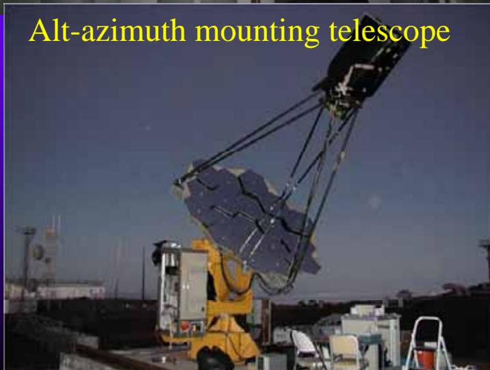
Alt-azimuth mounting telescope
