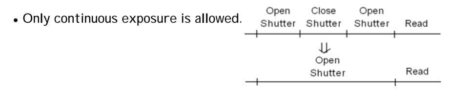
Pipeline operation is possible, but shutter must be open until previous readout is finished.
