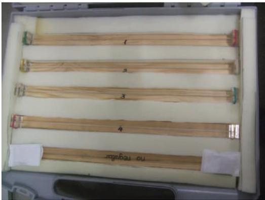
Fig. 12. Delivered sapphire fibers for KAGRA sapphire suspension
