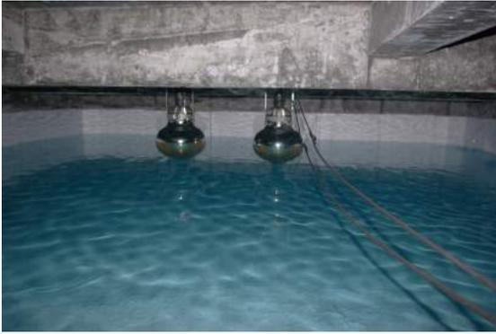
Fig. 25. PMTs mounted in a MD cell filled with water.
