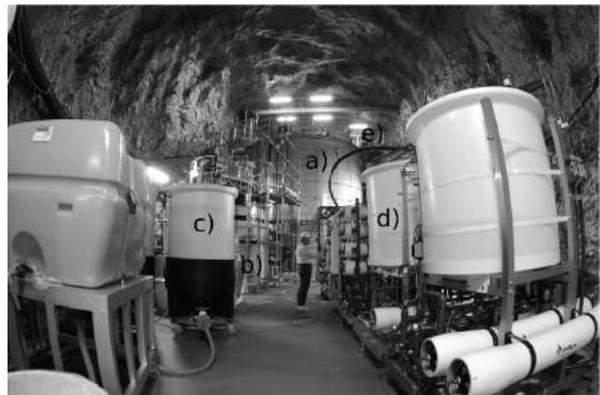
Fig. 23. In the new cavern the 200-ton tank (a) with currently 240 photomultipliers installed, the Gd pre-mixing and pre-treatment 15-ton tank (b), the selective filtration system (d), Gd removal resins (c) for test and a device to measure the water transparency (e) have been installed.
