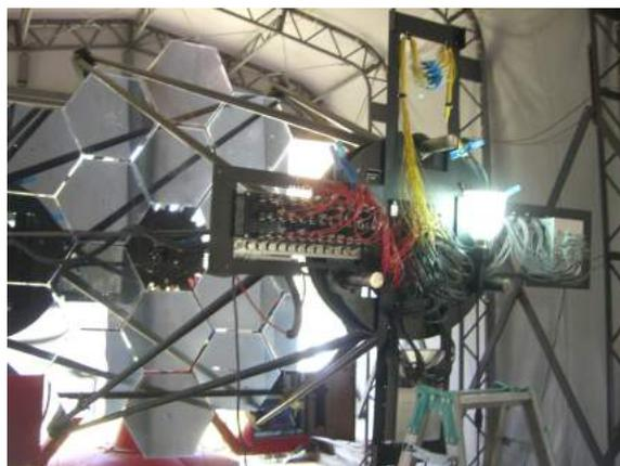
Fig. 6. Akeno atmospheric Cherenkov telescope equipped with an R & D system of 32 pixel imaging camera.
