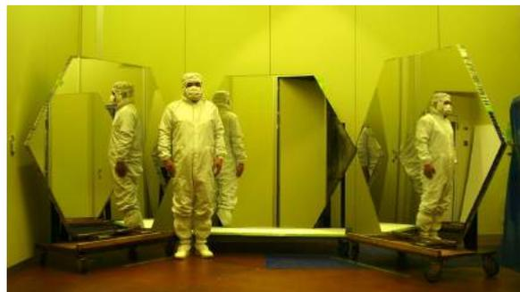
Fig. 4. The high precision segmented mirrors for the Large Size Telescope (LST) developed by CTA-Japan in cooperation with Sanko Co.LTD. The mirror is made of a 60mm thick aluminum honeycomb sandwiched by 3mm thin glass on both sides. A surface protection coat consisting of the materials SiO<sub>2</sub> and HfO<sub>2</sub> is applied to enhance the reflectivity and to elongate the lifetime.
