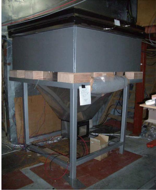
Fig. 3.  $0.5\text{-m}^2$  plastic scintillation counter for a new neutron telescope.
