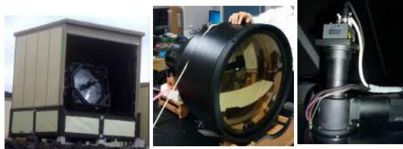
Fig. 34. Ashra-1 light collector (left), photo-electric lens imaging tube fabricated in 2016 (center) and photoelectric image pipeline (right).
