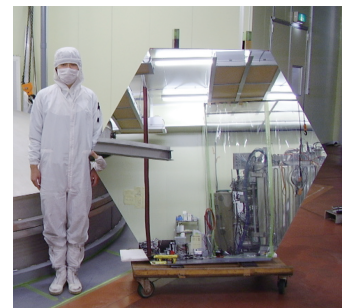
Fig. 5 Camera cluster for the Large Size Telescope (LST) developed by CTA-Japan. This cluster consists of seven high quantum efficiency photomultipliers (R1192Q-100), CW High Voltages, pre-amplifier, Slow Control Board, DRS4 Ultra fast waveform recording system and Trigger. The LST camera can be assembled with 400 of these clusters, cooling plates and camera housing.
