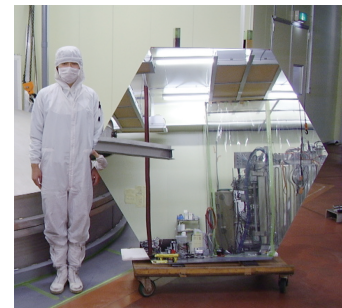
Fig. 5 Camera cluster for the Large Size Telescope (LST) developed by CTA-Japan. This cluster consists of seven high quantum efficiency photomultipliers (R11920-100), CW High Voltages, pre-amplifier, Slow Control Board, DRS4 Ultra fast waveform recording system and Trigger. The LST camera can be assembled with 400 of these clusters, cooling plates and camera housing.
