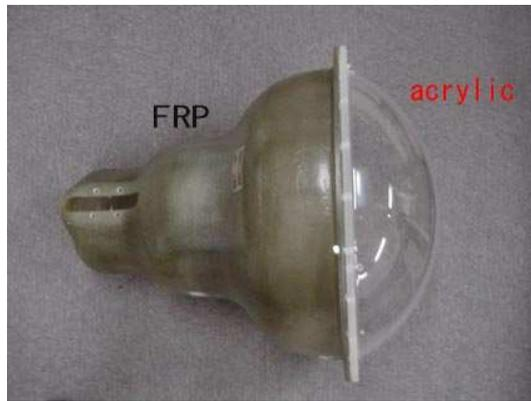
Figure 2.8: PMT case attached to the inner PMT after SK-II experiment
