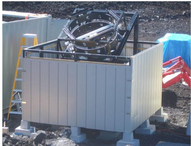
Fig. 14. Photograph of an Ashra light collector installed in a shelter. A motorized aluminum rolling door is equipped on the roof. Under the rolling door, an acrylic plate is placed over a 1,800-mm-square window.
