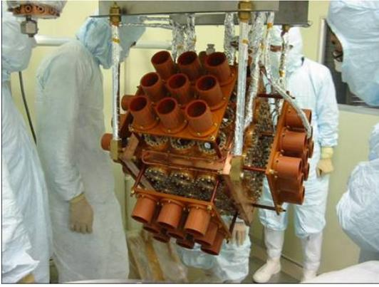
Fig. 2. 3 kg fiducial volume liquid xenon detector constructed for R&D study
