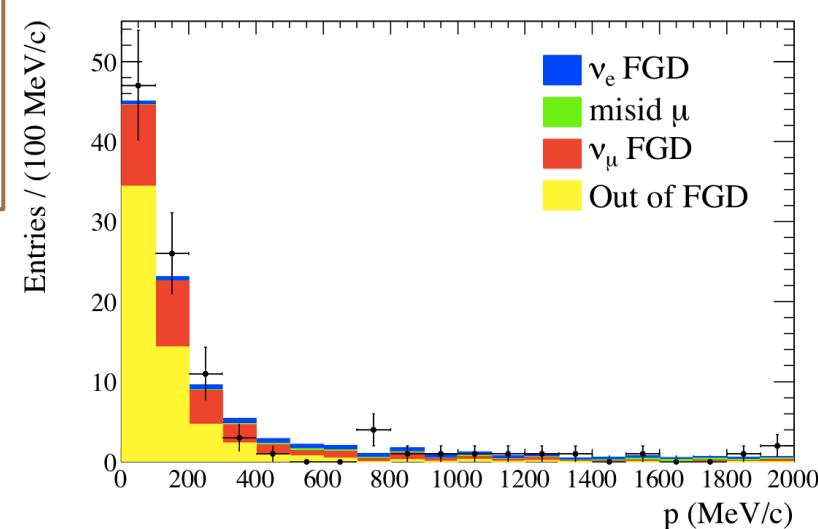
Data consistent with MC based on NA61 data and  $\nu$  interaction simulation
