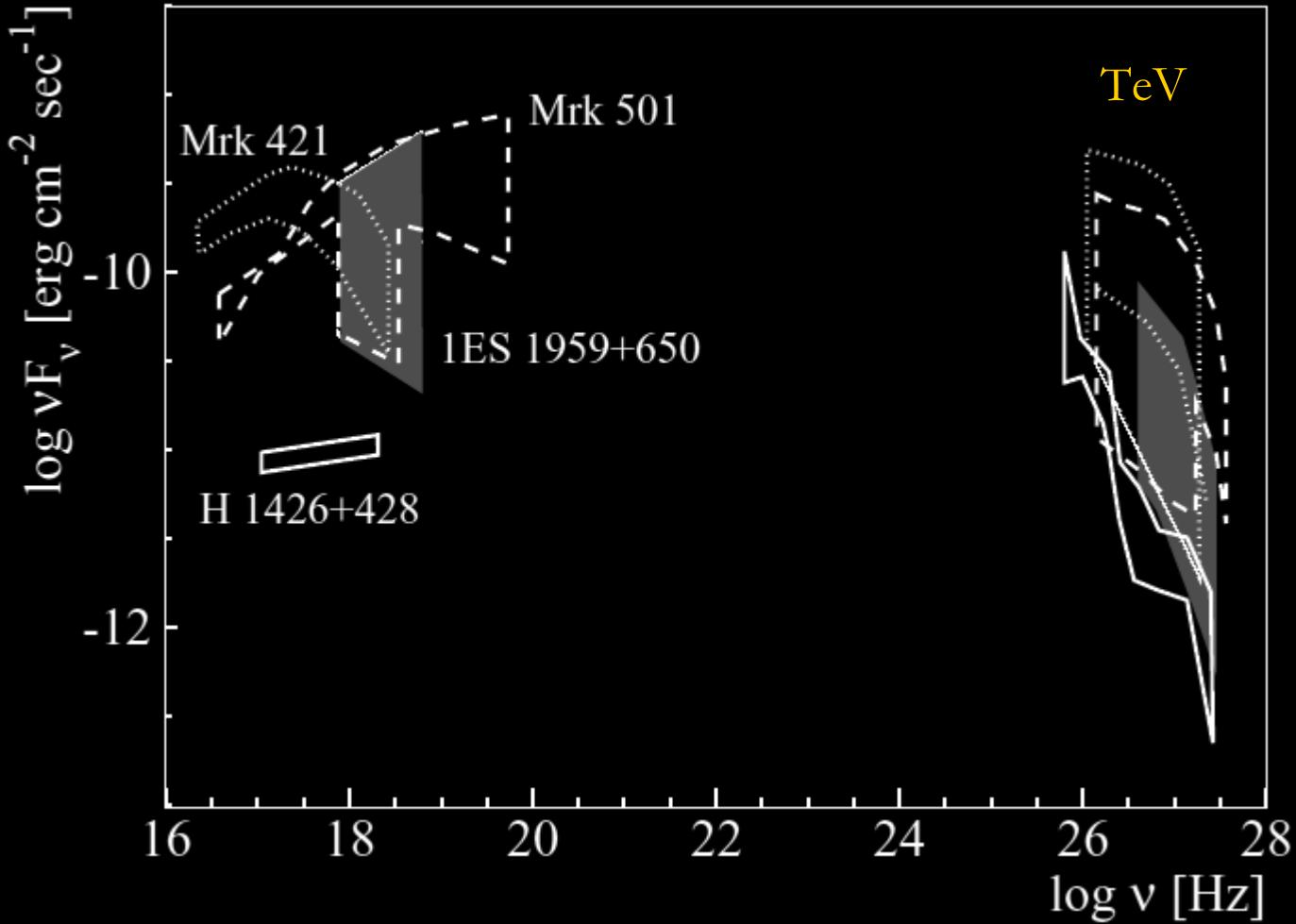
Fig. 1. Simultaneous and non-simultaneous X-ray and TeV  $\gamma$ -ray energy spectra of the 4 TeV blazars with measured TeV  $\gamma$ -ray energy spectra. The regions show the range of values that have been observed with BeppoSAX, RXTE and Cherenkov Telescopes (from (46)).
