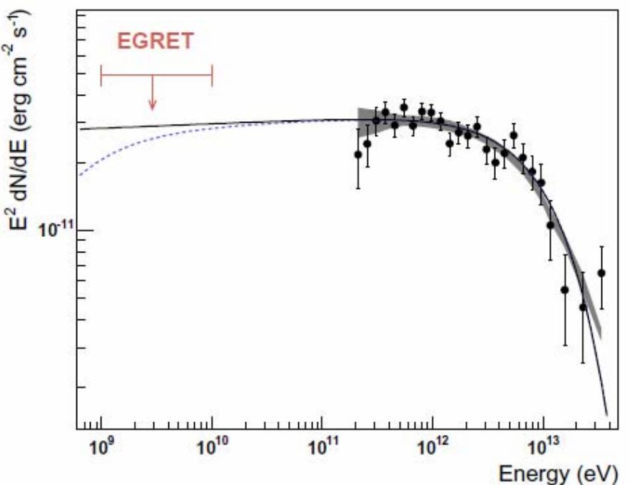
**Fig. 20.** H.E.S.S. data points plotted in an energy flux diagram. They shaded grey band is the systematic error band for this measurement (see Sect. 3.2). The black curve is the best fit of a power law with exponential cutoff to the data, extrapolated to lower energies. The dashed blue curves is the same function, but it takes the  $\pi^0$  kinematics into account. The EGRET upper limit from 1 GeV to 10 GeV is plotted as red arrow.
