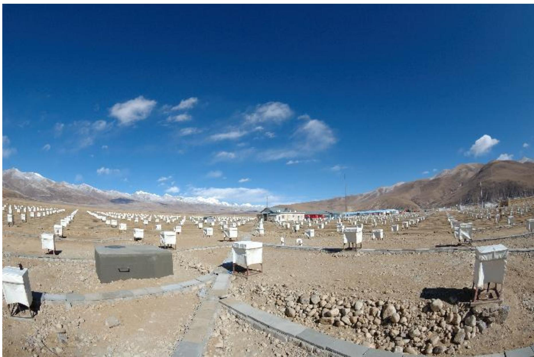
Prototype Muon Detector after backfilling
