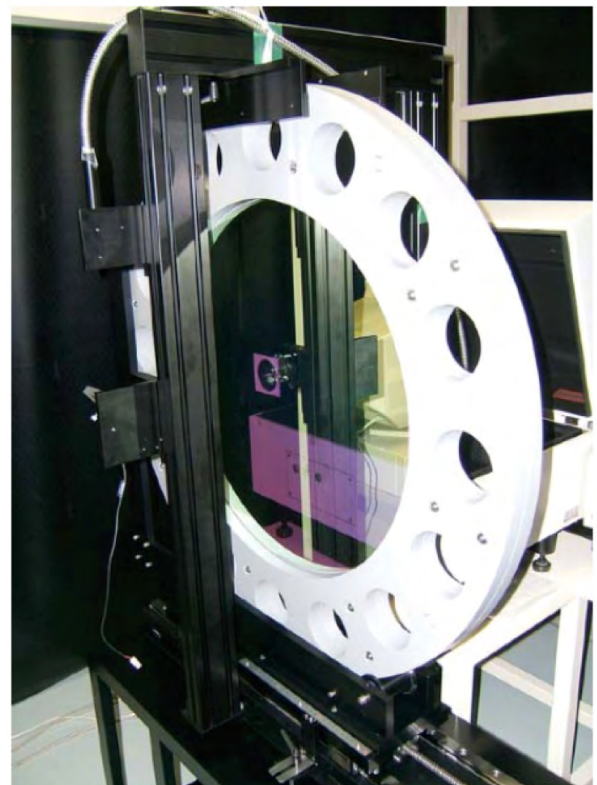
図6 開発中のすばる HSC 用狭帯域フィルター (Materion [旧 Barr Associates] 社と協力)。 Subaru/HSC narrow band filter under development (collaboration with Barr Associates Inc.)
