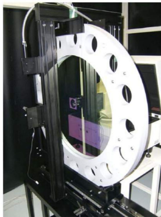
6 開発中のすばる HSC 用狭帯域フィルター (Materion [旧 Barr Associates] 社と協力)。 Subaru/HSC narrow band filter under development (collaboration with Barr Associates Inc.)
