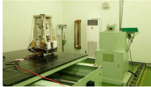
Fig. 41. Test at the high-dose facility of Fuji Electric Co. The detector was located at left and RI was located inside the heavy shield (light green, left).
