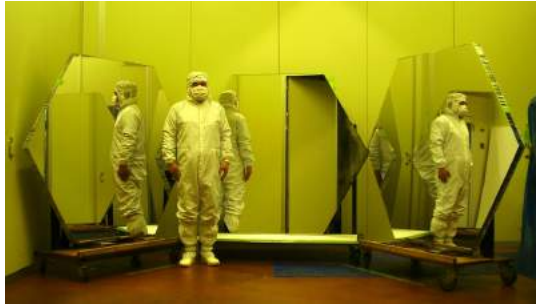
Fig. 4. The high precision segmented mirrors for the Large Size Telescope (LST) developed by CTA-Japan in cooperation with Sanko Co.LTD. The mirror is made of a 60mm thick aluminum honeycomb sandwiched by 3mm thin glass on both sides. A surface protection coat consisting of the materials SiO 2 and HfO 2 is applied to enhance the reflectivity and to elongate the lifetime.
