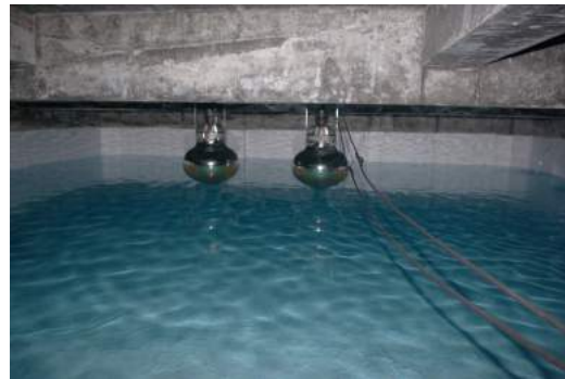
Fig. 26. PMTs mounted in a MD cell filled with water.
