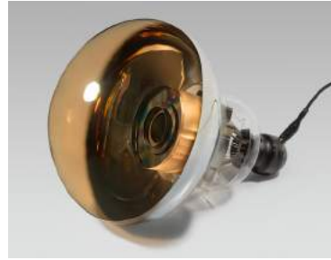
Fig. 42. New 50 cm photomultiplier tube with a box-and-line dynode (R12860, Hamamatsu Photonics K.K.).
