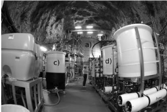
Fig. 19. In the new cavern, the 200-ton tank (a) with currently 240 photomultipliers installed, the Gd pre-mixing and pre-treatment 15-ton tank (b), the selective filtration system (d), Gd removal resins (c) for test and a device to measure the water transparency (e) have been installed.
