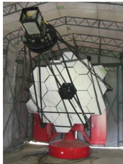
Fig. 6. Akeno atmospheric Cherenkov telescope of 3 m diameter, located in the Akeno Observatory.
