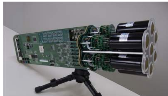
Fig. 3. Camera cluster for the Large Size Telescope (LST) developed by CTA-Japan. This cluster consists of seven high quantum efficiency photomultipliers (R11920-100), CW High Voltages, pre-amplifier, Slow Control Board, DRS4 Ultra fast waveform recording system and Trigger. The LST camera can be assembled with 265 of these clusters, cooling plates and camera housing.
