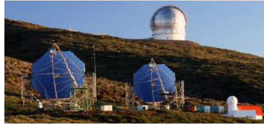
Fig. 5. MAGIC Stereo System with two Cherenkov telescopes of 17m diameters, so far achieved the threshold energy of 25GeV. It locates near the mountain top of the Roque de los Muchachos on the Canary Island of La Palma. Two telescopes are located with the distance of 85 meters.
