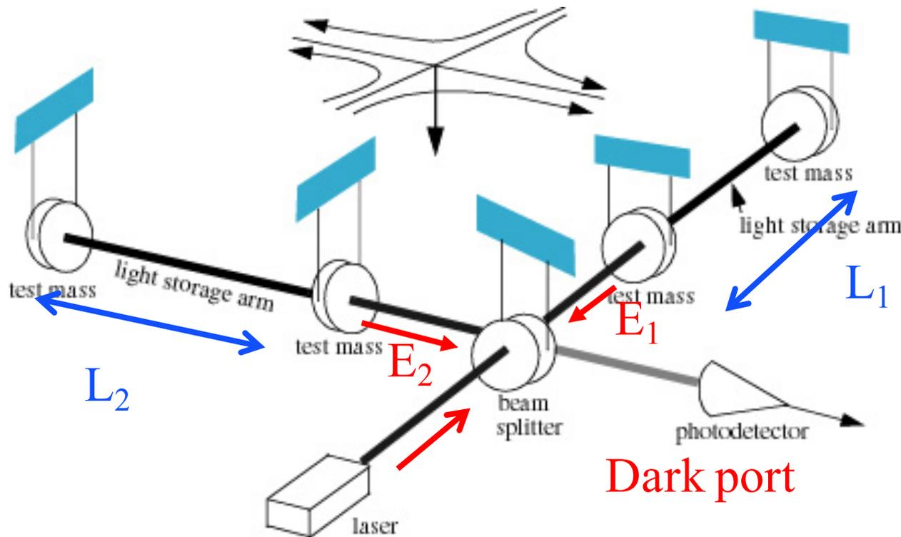
2 mirrors in the arm effectively lengthen the arm by  $\sim 1000$
