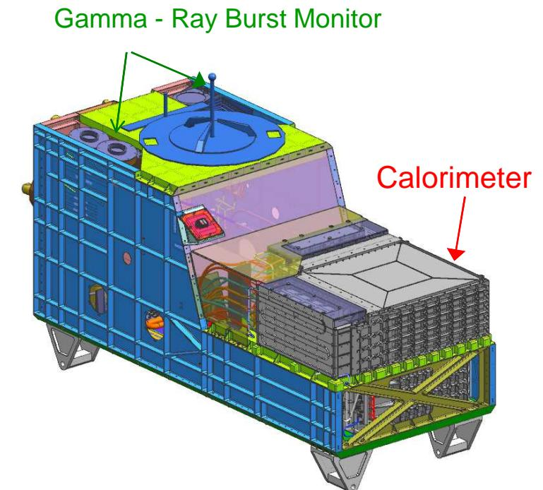
The CALET payload is launched by the Japanese carrier, H-II Transfer Vehicle 5 (HTV5) and robotically attached to the port #9 of the Japanese Experiment Module – Exposed Facility (JEM-EF) on the International Space Station.
