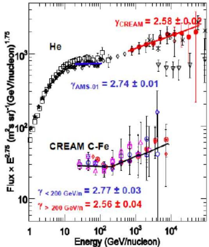
CALET will be able to perform an **accurate scan** of the energy region around the spectral break with an energy resolution  $\sim 30\%$  and larger GF  $\sim 0.1 \text{ m}^2 \text{ sr}$
