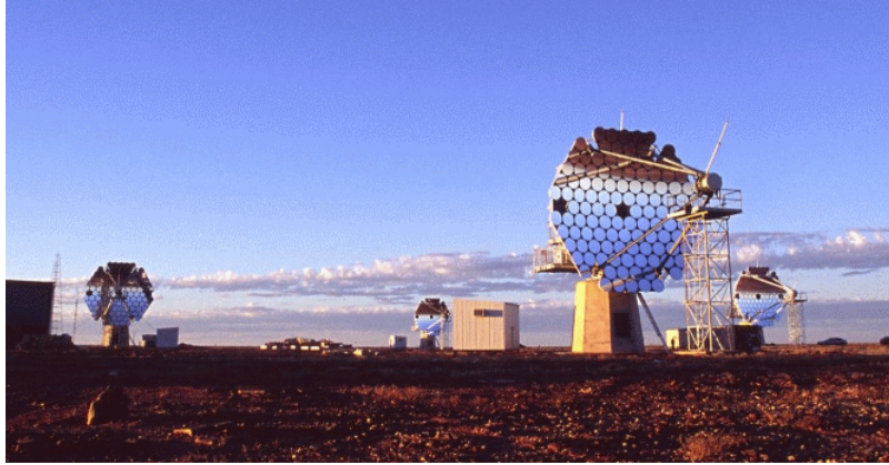
Figure 1: The CANGAROO-III system of telescopes as of March 2004. The telescope seen at right is the CANGAROO-II.
