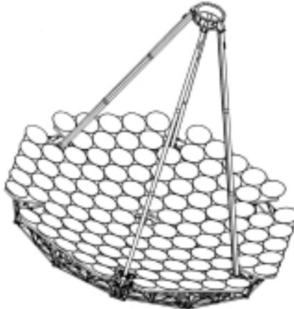
**FIGURE 2.** A sketch of the 10 m reflector.
