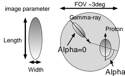
Fig. 13. Schematic view describing the parameterization in imaging air Čerenkov technique.
