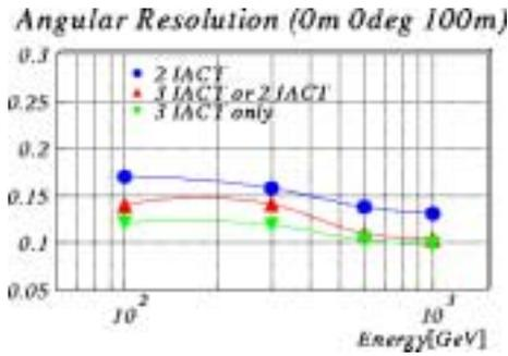
Fig. 16. Simulated performances of the angular resolution of the stereo observation using several 10m IACTs designed for CANGAROO-III.
