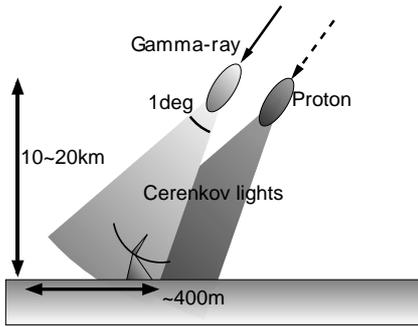
Fig. 12. Schematic image describing the principle of air Čerenkov technique.
