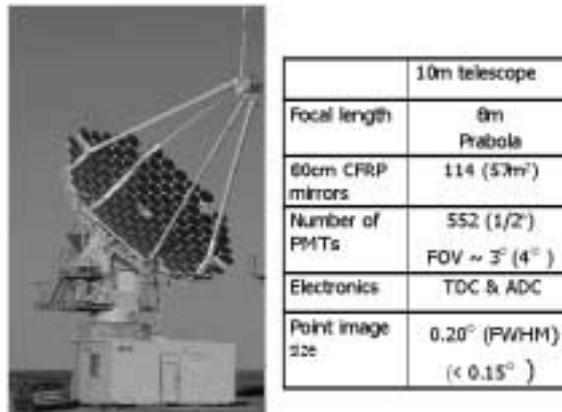
Fig. 18. The 10 m telescope completed in February 2000 in Woomera, South Australia.
