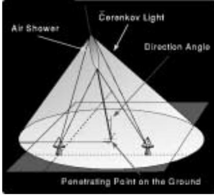
Fig. 14. Schematic diagram describing the principle of stereo observation.
