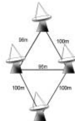
Fig. 19. Arrangement of the array of CANGAROO-III four telescopes.
