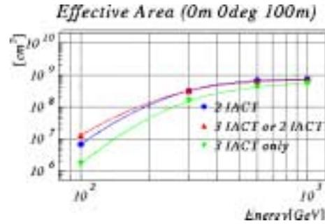
Fig. 17. Simulated performances of the effective area of the stereo observation using several 10m IACTs designed for CANGAROO-III.
