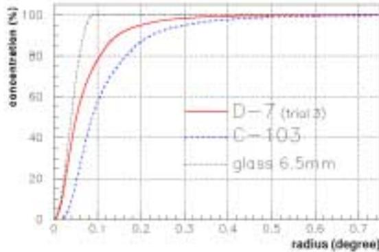
Figure 4: Concentration ratios of light on the focus as a function of radius for glass mirror(dotted), plastic mirror that is being developed (solid) and plastic mirror used in the 1st telescope (broken).
