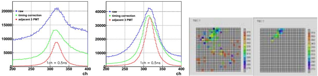
Figure 2: On (1st from the left) and Off (2nd) Timing distributions of all hit PMTs in cases of raw data (top line), after corrections of time walk and the timing center of each event (middle), and after requirement of at least 3 adjacent hit PMTs(bottom). Also images on the camera before (3rd) and after the noise reduction (4th) are presented.
