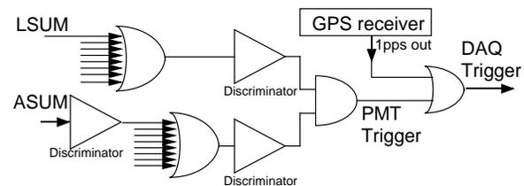
Fig. 3. DAQ trigger of the first telescope.
