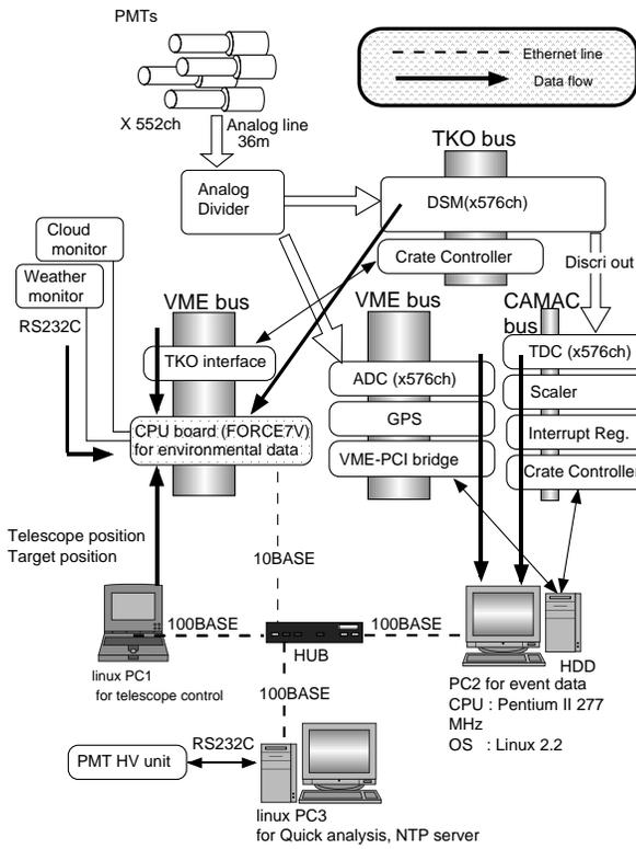
Fig. 1. Overview of data acquisition system of the first telescope.
