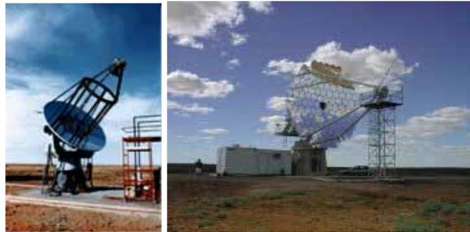
**Fig. 1.** CANGAROO-I telescope(left) and CANGAROO-II telescope(right). Mirror diameters are 3.8m(left) and 10m(right), respectively.
