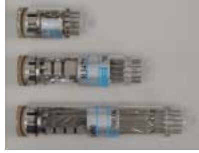
Fig. 3. Performance tests were made for three types of 19mm (3/4 inch) diameter photomultiplier tubes (PMTs). The model numbers are, from top to bottom, Hamamatsu Photonics R5611, R3479 and R1450, respectively. The R3479 was selected for the CANGAROO-III PMT module.
