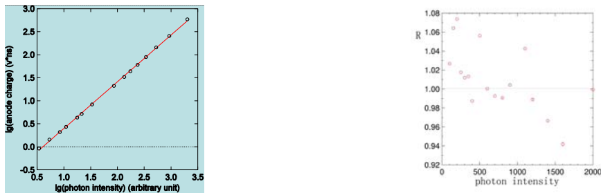
Figure 3. The linearity of the PMT over a range from a few pe's to thousands pe's.
