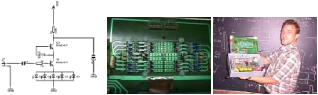
Fig. 2. The functionalities of the pulser board: A circuit of two avalanche transistors discharges a small capacitance charged with 600V through five parallel LEDs providing an ultra-short (3–4 ns) and powerful light pulse. The pulser board integrates 16 of such circuits housing LEDs in one of the three colours: green, blue and UV. The pulser board and steering electronics (right) (500 MHz bandwidth GaAs analog switch controlled by CAN bus). The LED slots can be switched on and off individually thus allowing for different intensities and colours. The light uniformity at the camera is around 2–3%.
