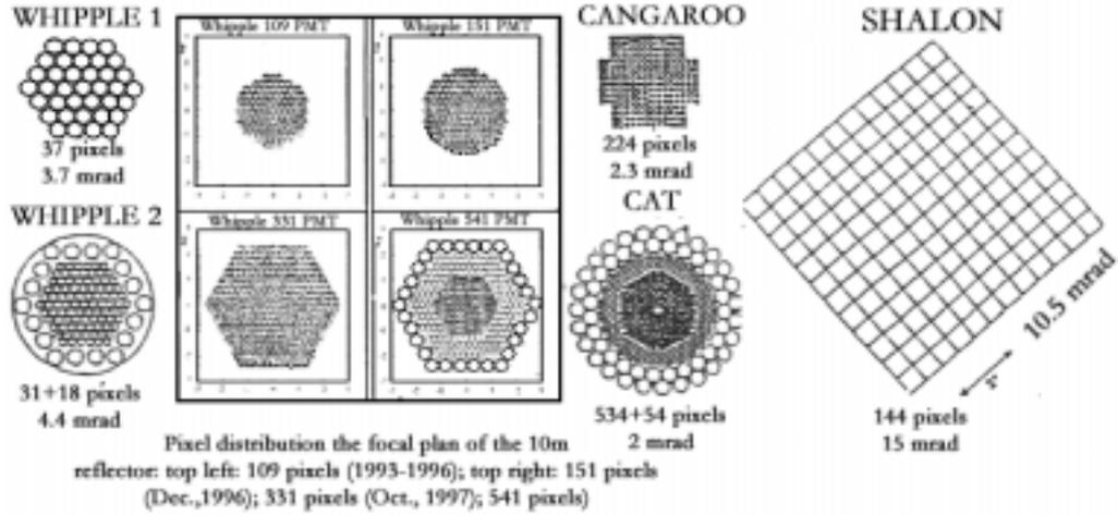
**Fig. 2.** Evolution of PMT arrays to record images seen in Cherenkov light.
