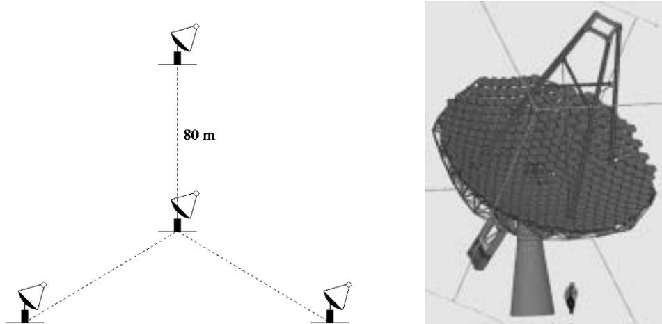
**Fig. 1.** Layout of telescopes for VERITAS-4 (left). Three additional reflectors will be added to complete the full array of seven telescopes. Design of optical support structure for each 12 m telescope (right).
