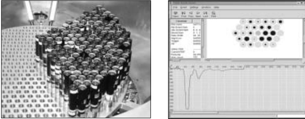
**Fig. 2.** Camera integration for prototype VERITAS telescope, partially completed (left). Display from FADC sampling of Cherenkov pulse (right). The second peak corresponds to a delayed copy of the pulse with lower gain.
