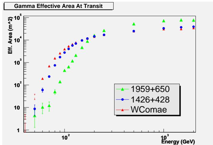
**Fig. 3.** Effective areas of the STACEE detector for gamma-rays as a function of energy for three sources observed by STACEE as calculated using a Monte Carlo.
