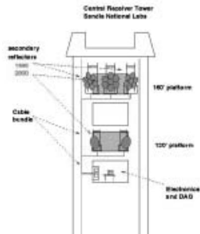
**Fig. 2.** Sketch of the tower at the NSTTF showing the positions of the STACEE secondary mirrors.
