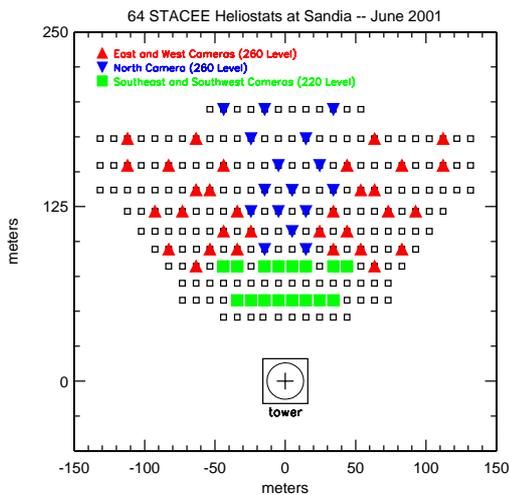
**Fig. 1.** Map of the National Solar Thermal Test Facility (NSTTF) showing the heliostats used by STACEE.
