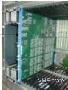
Custom-built VME-base front-end module
