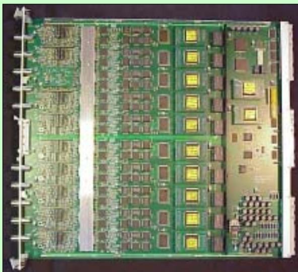
Completed FADC Board 10 chans, 9U VME
