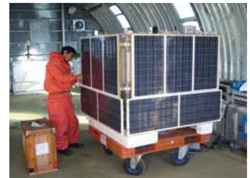
PPB-BETS with solar panels
