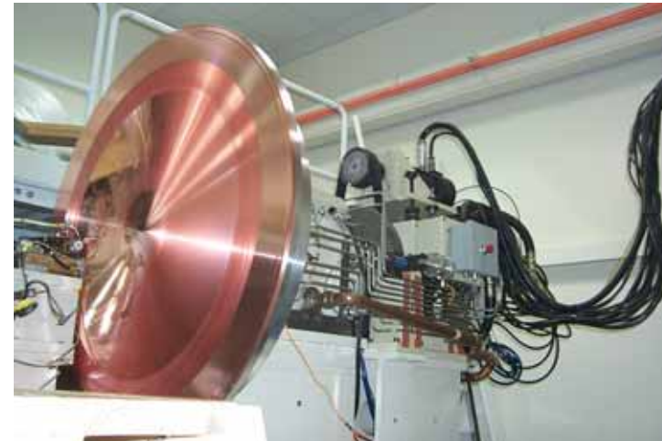
Fresnel lens 1.5 m diameter.
